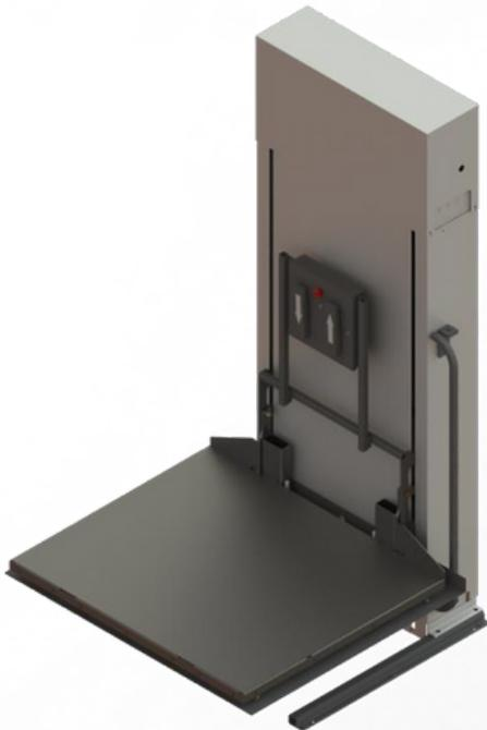
2) Lower the platform as shown and tighten the platform mounting bolts (1/2" bolts). Check that the emergency stop button is not depressed and that the on/off key is in and turned clockwise. Plug the lift into the wall outlet (standard 110V 15A outlet). Test the lift operation by pressing the up and down paddles.
