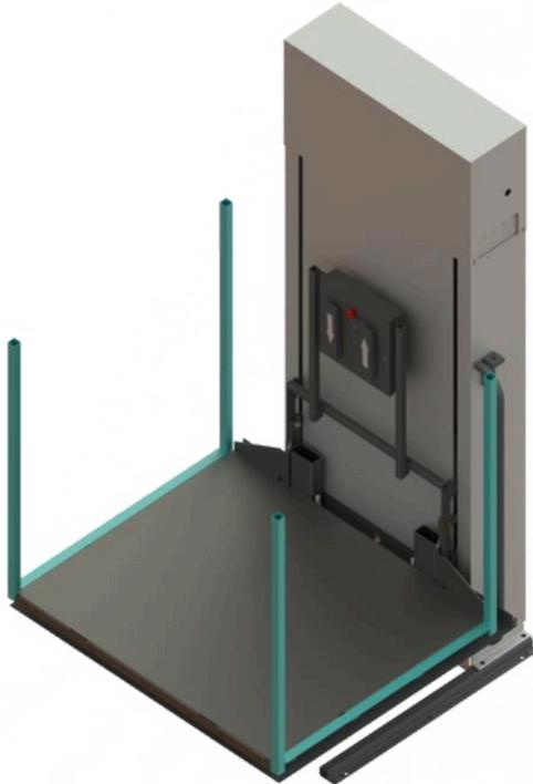
3) Attach 1 1/2" extension weldments to the lift platform using 5/16" hex head screws, washers and lock nuts.
