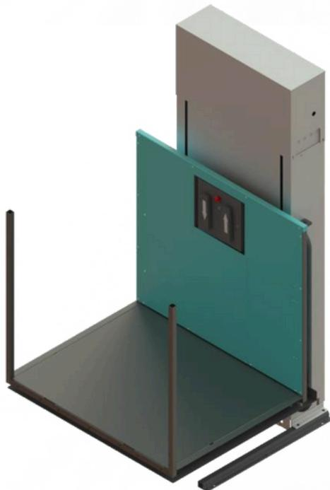
4) Attach the handrail top and bottom tubes to the platform handrail control wall using 3/16" rivets. Add plugs to the top handrail tube. Attach the platform handrail control wall to 1 1/2" extension weldment posts using 3/16" rivets. Attach the inspection/maintenance panel to the platform handrail control panel using #10-24 screws.
