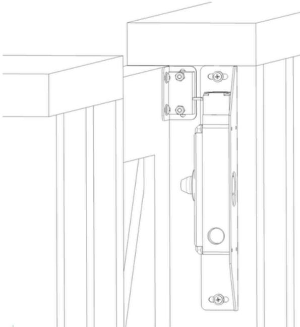
To begin, ensure the gate is in the closed position. Confirm the tab and bracket assembly is inserted into the interlock, and position it near the top of the gate to get the approximate alignment of the tab and lock. The mounting brackets are slotted to provide three-axis adjustability.
