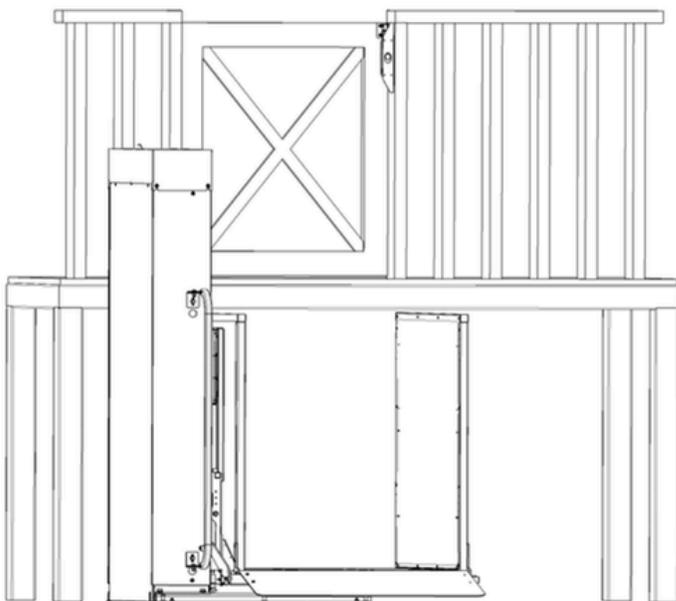
Interlocks are designed to ensure that landing doors and gates remain securely closed when the lift is not at that landing. This safety mechanism prevents the doors from opening and provides a secure barrier, maintaining proper operational safety and preventing unauthorized access to the lift shaft.
