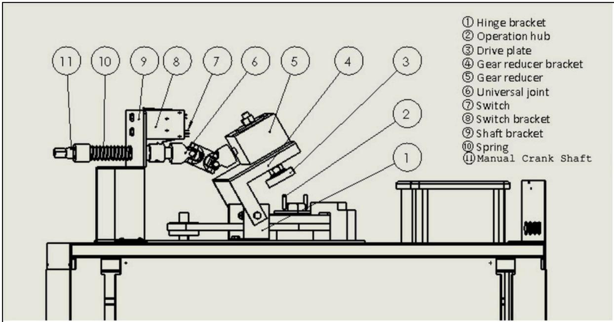
The above figure shows the normal position of the 90 Degree Manual Crank, disengaged. While the figure only shows the manual crank access on the left, the side the crank is on is specified at the time of order.
