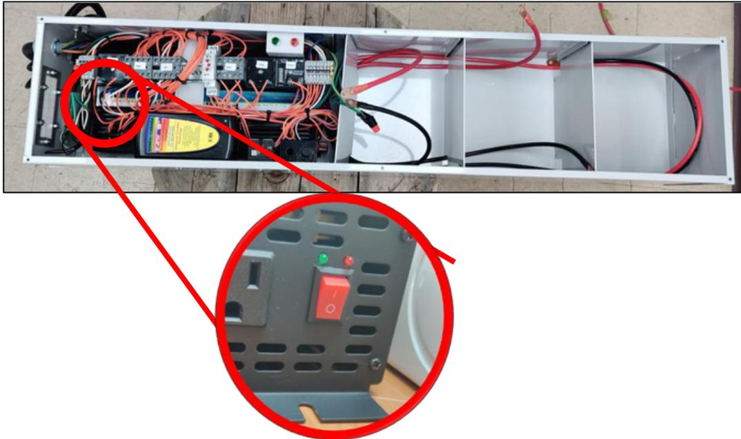
6) Wait 105 seconds, and battery power light should come on. Once you confirm that the tower is operating correctly, reinstall the front cover.
