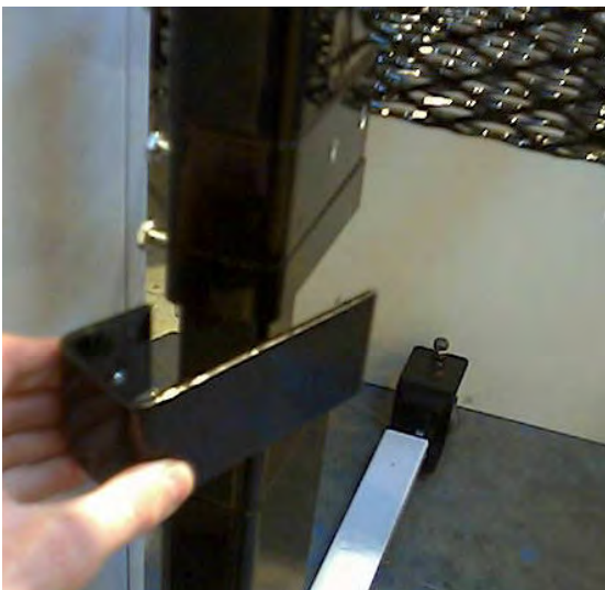
FIG.18-REMOVE ANY UNNECESSARY SPACERS
